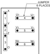
Figure 18. Voltage Change-Over Board 240V Configuration
